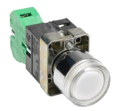
AutomationDirect pushbutton, IP65, 22mm, momentary, incandescent illuminated, (1) N.O. contact(s), metal base, metal bezel, plastic ring, Operator: clear, flush, 30mm, round, plastic, 120 VAC/VDC, full voltage.
