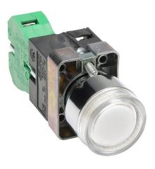
AutomationDirect pushbutton, IP65, 22mm, momentary, LED illuminated, (1) N.O. contact(s), metal base, metal bezel, plastic ring, Operator: clear, flush, 30mm, round, plastic, 120 VAC/VDC, full voltage.
