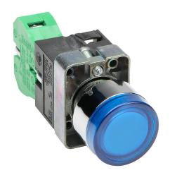
AutomationDirect pushbutton, IP65, 22mm, momentary, LED illuminated, (1) N.O. contact(s), metal base, metal bezel, plastic ring, Operator: blue, flush, 30mm, round, plastic, 24 VAC/VDC, full voltage.
