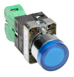
AutomationDirect pushbutton, IP65, 22mm, momentary, LED illuminated, (1) N.O. contact(s), metal base, metal bezel, plastic ring, Operator: blue, flush, 30mm, round, plastic, 120 VAC/VDC, full voltage.
