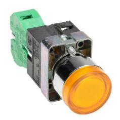
AutomationDirect pushbutton, IP65, 22mm, momentary, incandescent illuminated, (1) N.O. contact(s), metal base, metal bezel, plastic ring, Operator: yellow, flush, 30mm, round, plastic, 24 VAC/VDC, full voltage.
