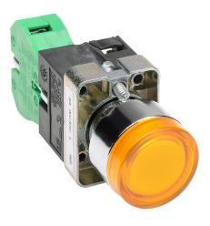
AutomationDirect pushbutton, IP65, 22mm, momentary, LED illuminated, (1) N.O. contact(s), metal base, metal bezel, plastic ring, Operator: yellow, flush, 30mm, round, plastic, 24 VAC/VDC, full voltage.
