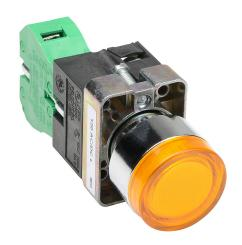
AutomationDirect pushbutton, IP65, 22mm, momentary, LED illuminated, (1) N.O. contact(s), metal base, metal bezel, plastic ring, Operator: yellow, flush, 30mm, round, plastic, 120 VAC/VDC, full voltage.
