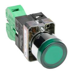
AutomationDirect pushbutton, IP65, 22mm, momentary, incandescent illuminated, (1) N.O. contact(s), metal base, metal bezel, plastic ring, Operator: green, flush, 30mm, round, plastic, 24 VAC/VDC, full voltage.
