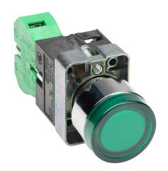
AutomationDirect pushbutton, IP65, 22mm, momentary, LED illuminated, (1) N.O. contact(s), metal base, metal bezel, plastic ring, Operator: green, flush, 30mm, round, plastic, 24 VAC/VDC, full voltage.
