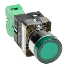
AutomationDirect pushbutton, IP65, 22mm, momentary, incandescent illuminated, (1) N.O. contact(s), metal base, metal bezel, plastic ring, Operator: green, flush, 30mm, round, plastic, 120 VAC/VDC, full voltage.
