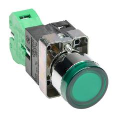
AutomationDirect pushbutton, IP65, 22mm, momentary, LED illuminated, (1) N.O. contact(s), metal base, metal bezel, plastic ring, Operator: green, flush, 30mm, round, plastic, 120 VAC/VDC, full voltage.
