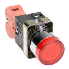
AutomationDirect pushbutton, IP65, 22mm, momentary, incandescent illuminated, (1) N.C. contact(s), metal base, metal bezel, plastic ring, Operator: red, flush, 30mm, round, plastic, 24 VAC/VDC, full voltage.
