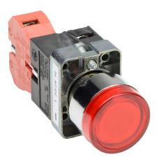
AutomationDirect pushbutton, IP65, 22mm, momentary, LED illuminated, (1) N.C. contact(s), metal base, metal bezel, plastic ring, Operator: red, flush, 30mm, round, plastic, 24 VAC/VDC, full voltage.
