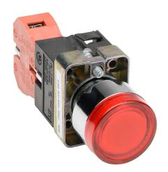
AutomationDirect pushbutton, IP65, 22mm, momentary, incandescent illuminated, (1) N.C. contact(s), metal base, metal bezel, plastic ring, Operator: red, flush, 30mm, round, plastic, 120 VAC/VDC, full voltage.
