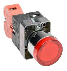
AutomationDirect pushbutton, IP65, 22mm, momentary, LED illuminated, (1) N.C. contact(s), metal base, metal bezel, plastic ring, Operator: red, flush, 30mm, round, plastic, 120 VAC/VDC, full voltage.
