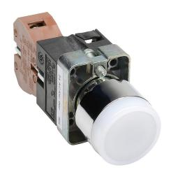
AutomationDirect pushbutton, IP65, 22mm, push ON - push OFF, incandescent illuminated, (1) N.O. contact(s), metal base, metal bezel, plastic ring, Operator: white, flush, 30mm, round, plastic, 24 VAC/VDC, full voltage.
