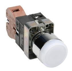
AutomationDirect pushbutton, IP65, 22mm, push ON - push OFF, LED illuminated, (1) N.O. contact(s), metal base, metal bezel, plastic ring, Operator: white, flush, 30mm, round, plastic, 24 VAC/ VDC, full voltage.
