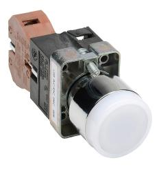
AutomationDirect pushbutton, IP65, 22mm, push ON - push OFF, incandescent illuminated, (1) N.O. contact(s), metal base, metal bezel, plastic ring, Operator: white, flush, 30mm, round, plastic, 120 VAC/VDC, full voltage.
