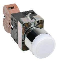
AutomationDirect pushbutton, IP65, 22mm, push ON - push OFF, LED illuminated, (1) N.O. contact(s), metal base, metal bezel, plastic ring, Operator: white, flush, 30mm, round, plastic, 120 VAC/ VDC, full voltage.
