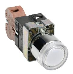
AutomationDirect pushbutton, IP65, 22mm, push ON - push OFF, incandescent illuminated, (1) N.O. contact(s), metal base, metal bezel, plastic ring, Operator: clear, flush, 30mm, round, plastic, 120 VAC/VDC, full voltage.
