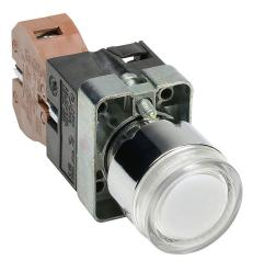
AutomationDirect pushbutton, IP65, 22mm, push ON - push OFF, LED illuminated, (1) N.O. contact(s), metal base, metal bezel, plastic ring, Operator: clear, flush, 30mm, round, plastic, 120 VAC/ VDC, full voltage.
