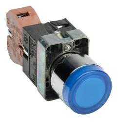
AutomationDirect pushbutton, IP65, 22mm, push ON - push OFF, incandescent illuminated, (1) N.O. contact(s), metal base, metal bezel, plastic ring, Operator: blue, flush, 30mm, round, plastic, 24 VAC/VDC, full voltage.
