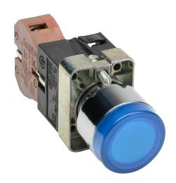
AutomationDirect pushbutton, IP65, 22mm, push ON - push OFF, LED illuminated, (1) N.O. contact(s), metal base, metal bezel, plastic ring, Operator: blue, flush, 30mm, round, plastic, 24 VAC/ VDC, full voltage.
