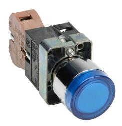
AutomationDirect pushbutton, IP65, 22mm, push ON - push OFF, incandescent illuminated, (1) N.O. contact(s), metal base, metal bezel, plastic ring, Operator: blue, flush, 30mm, round, plastic, 120 VAC/VDC, full voltage.
