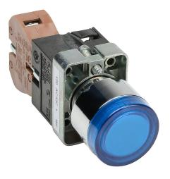
AutomationDirect pushbutton, IP65, 22mm, push ON - push OFF, LED illuminated, (1) N.O. contact(s), metal base, metal bezel, plastic ring, Operator: blue, flush, 30mm, round, plastic, 120 VAC/ VDC, full voltage.
