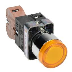
AutomationDirect pushbutton, IP65, 22mm, push ON - push OFF, incandescent illuminated, (1) N.O. contact(s), metal base, metal bezel, plastic ring, Operator: yellow, flush, 30mm, round, plastic, 24 VAC/VDC, full voltage.
