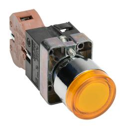
AutomationDirect pushbutton, IP65, 22mm, push ON - push OFF, LED illuminated, (1) N.O. contact(s), metal base, metal bezel, plastic ring, Operator: yellow, flush, 30mm, round, plastic, 24 VAC/VDC, full voltage.
