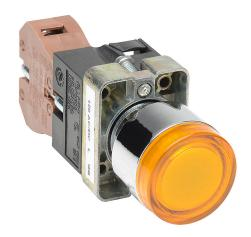
AutomationDirect pushbutton, IP65, 22mm, push ON - push OFF, LED illuminated, (1) N.O. contact(s), metal base, metal bezel, plastic ring, Operator: yellow, flush, 30mm, round, plastic, 120 VAC/VDC, full voltage.
