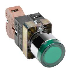
AutomationDirect pushbutton, IP65, 22mm, push ON - push OFF, incandescent illuminated, (1) N.O. contact(s), metal base, metal bezel, plastic ring, Operator: green, flush, 30mm, round, plastic, 24 VAC/VDC, full voltage.
