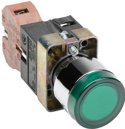
AutomationDirect pushbutton, IP65, 22mm, push ON - push OFF, incandescent illuminated, (1) N.O. contact(s), metal base, metal bezel, plastic ring, Operator: green, flush, 30mm, round, plastic, 24 VAC/VDC, full voltage.
