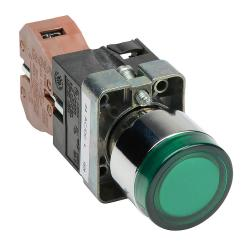
AutomationDirect pushbutton, IP65, 22mm, push ON - push OFF, LED illuminated, (1) N.O. contact(s), metal base, metal bezel, plastic ring, Operator: green, flush, 30mm, round, plastic, 24 VAC/ VDC, full voltage.
