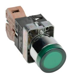
AutomationDirect pushbutton, IP65, 22mm, push ON - push OFF, LED illuminated, (1) N.O. contact(s), metal base, metal bezel, plastic ring, Operator: green, flush, 30mm, round, plastic, 120 VAC/VDC, full voltage.
