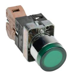
AutomationDirect pushbutton, IP65, 22mm, push ON - push OFF, LED illuminated, (1) N.O. contact(s), metal base, metal bezel, plastic ring, Operator: green, flush, 30mm, round, plastic, 120 VAC/VDC, full voltage.
