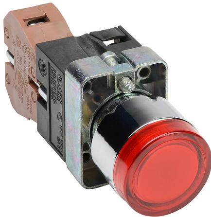
AutomationDirect pushbutton, IP65, 22mm, push ON - push OFF, incandescent illuminated, (1) N.O. contact(s), metal base, metal bezel, plastic ring, Operator: red, flush, 30mm, round, plastic, 24 VAC/VDC, full voltage.
