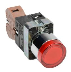
AutomationDirect pushbutton, IP65, 22mm, push ON - push OFF, incandescent illuminated, (1) N.O. contact(s), metal base, metal bezel, plastic ring, Operator: red, flush, 30mm, round, plastic, 24 VAC/VDC, full voltage.
