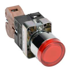
AutomationDirect pushbutton, IP65, 22mm, push ON - push OFF, LED illuminated, (1) N.O. contact(s), metal base, metal bezel, plastic ring, Operator: red, flush, 30mm, round, plastic, 24 VAC/ VDC, full voltage.
