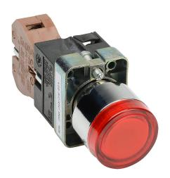
AutomationDirect pushbutton, IP65, 22mm, push ON - push OFF, incandescent illuminated, (1) N.O. contact(s), metal base, metal bezel, plastic ring, Operator: red, flush, 30mm, round, plastic, 120 VAC/VDC, full voltage.
