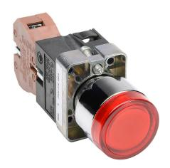
AutomationDirect pushbutton, IP65, 22mm, push ON - push OFF, LED illuminated, (1) N.O. contact(s), metal base, metal bezel, plastic ring, Operator: red, flush, 30mm, round, plastic, 120 VAC/VDC, full voltage.
