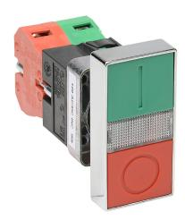
AutomationDirect pushbutton, IP65, 22mm, momentary, incandescent illuminated, (1) N.O./(1) N.C. contact(s), metal base, metal bezel, Operator: red/green, double headed, 50mm, rectangular, plastic, operator text "(I) and (0)", 120 VAC/VDC, full voltage.
