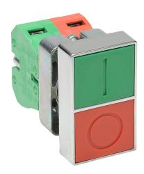
AutomationDirect pushbutton, IP65, 22mm, momentary, (1) N.O./ (1) N.C. contact(s), metal base, metal bezel, Operator: red/green, double headed, 50mm, rectangular, plastic, operator text "(I) and (0)".
