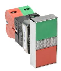
AutomationDirect pushbutton, IP65, 22mm, momentary, incandescent illuminated, (1) N.O./(1) N.C. contact(s), metal base, metal bezel, Operator: red/green, double headed, 60mm, rectangular, plastic, 24 VAC/VDC, full voltage.
