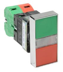
AutomationDirect pushbutton, IP65, 22mm, momentary, incandescent illuminated, (1) N.O./(1) N.C. contact(s), metal base, metal bezel, Operator: red/green, double headed, 60mm, rectangular, plastic, 120 VAC/VDC, full voltage.
