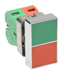
AutomationDirect pushbutton, IP65, 22mm, momentary, (1) N.O./ (1) N.C. contact(s), metal base, metal bezel, Operator: red/green, double headed, 60mm, rectangular, plastic.
