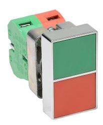
AutomationDirect pushbutton, IP65, 22mm, momentary, (1) N.O./ (1) N.C. contact(s), metal base, metal bezel, Operator: red/green, double headed, 50mm, rectangular, plastic.
