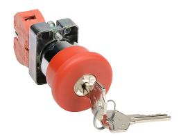
AutomationDirect emergency stop pushbutton, IP65, 22mm, key operated release, (1) N.C. contact(s), metal base, metal bezel, Operator: red, mushroom, 40mm, round, plastic.
