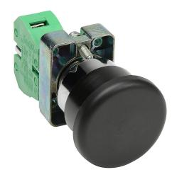
AutomationDirect pushbutton, IP65, 22mm, momentary, (1) N.O. contact(s), metal base, metal bezel, Operator: black, mushroom, 40mm, round, plastic.
