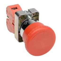
AutomationDirect emergency stop pushbutton, IP65, 22mm, twist-to-release, (1) N.C. contact(s), metal base, metal bezel, Operator: red, mushroom, 40mm, round, plastic.
