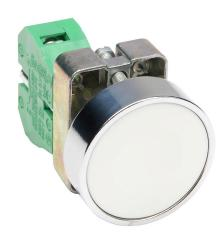
AutomationDirect pushbutton, IP65, 22mm, momentary, (1) N.O. contact(s), metal base, metal bezel, Operator: white, flush, 40mm, round, plastic.
