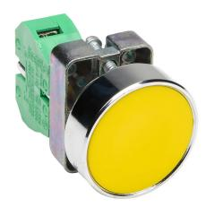
AutomationDirect pushbutton, IP65, 22mm, momentary, (1) N.O. contact(s), metal base, metal bezel, Operator: yellow, flush, 40mm, round, plastic.
