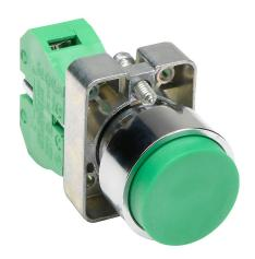
AutomationDirect pushbutton, IP65, 22mm, momentary, (1) N.O. contact(s), metal base, metal bezel, Operator: green, extended, 30mm, round, plastic.
