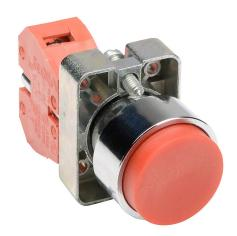
AutomationDirect pushbutton, IP65, 22mm, momentary, (1) N.C. contact(s), metal base, metal bezel, Operator: red, extended, 30mm, round, plastic.
