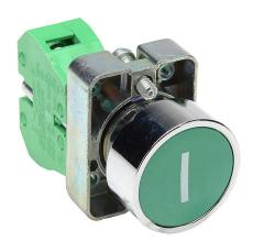
AutomationDirect pushbutton, IP65, 22mm, momentary, (1) N.O. contact(s), metal base, metal bezel, Operator: green, flush, 30mm, round, plastic, operator text "(I)".
