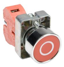
AutomationDirect pushbutton, IP65, 22mm, momentary, (1) N.C. contact(s), metal base, metal bezel, Operator: red, flush, 30mm, round, plastic, operator text "(O)".
