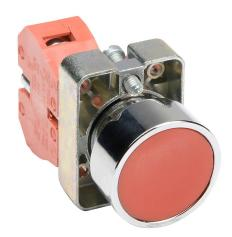
AutomationDirect pushbutton, IP65, 22mm, momentary, (1) N.C. contact(s), metal base, metal bezel, Operator: red, flush, 30mm, round, plastic.
